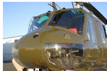
Figure 10 Flush mounted airspeed preproduction prototype on the OADS UH-1H.
