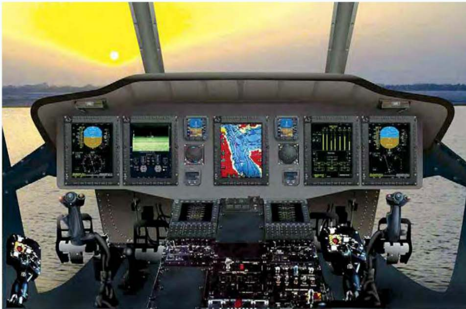
Rockwell Collins is fielding a brownout approach and hover symbology in its CAAS-equipped cockpits, such as this SOCOM MH-60. (Photo courtesy of Rockwell Collins.)
