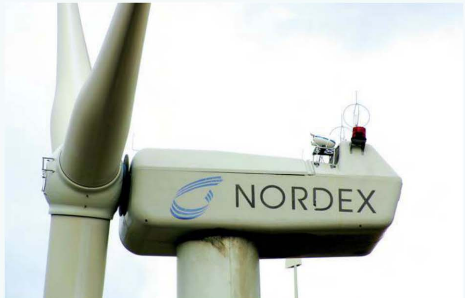
The Vindicator Laser Wind Sensor is being tested to provide wind turbine control based on wind ahead of the turbine blade. (Photo courtesy of OADS.)
