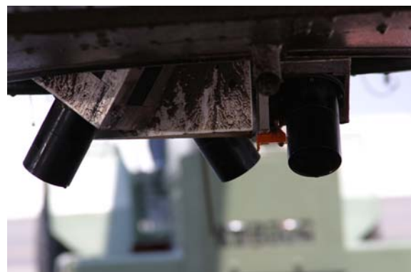
Figure 6 The groundspeed lens assemblies mounted on the OADS UH-1H following a dust test flight.
