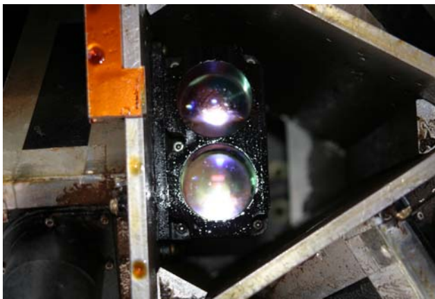
Figure 7 The laser altimeter sensor mounted on the OADS UH-1H. The lenses, coated with a layer of oil and dirt, remained functional throughout the flight test.
